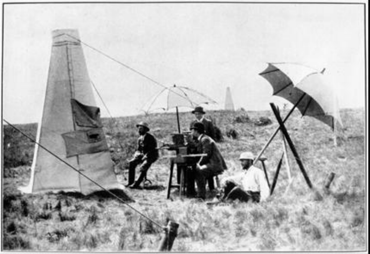
The first torsion balance field measurements carried out by Eötvös on Ság Hill of Transdanubia in August 1891 (courtesy of Eötvös Loránd Geophysical Institute)
